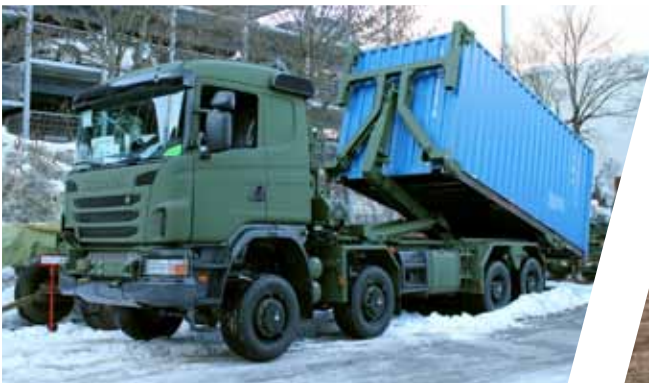
Load Handling system with CHU
