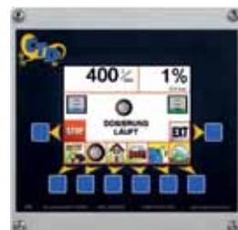
Monitor foaming agent admixing system
