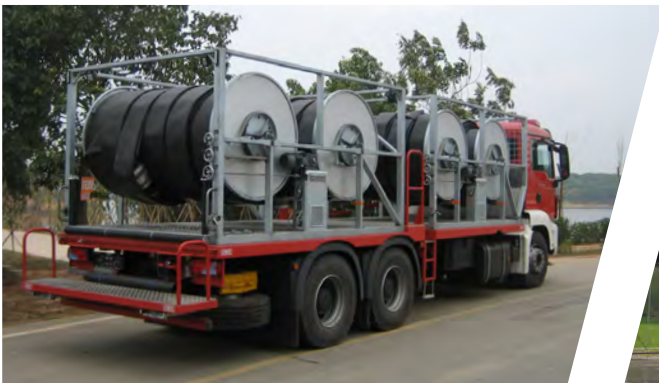
管道铺设车 Hose Laying Vehicle
