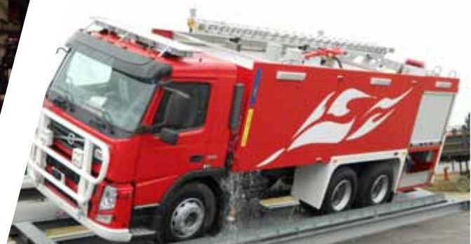
Kipptest Tipping test
